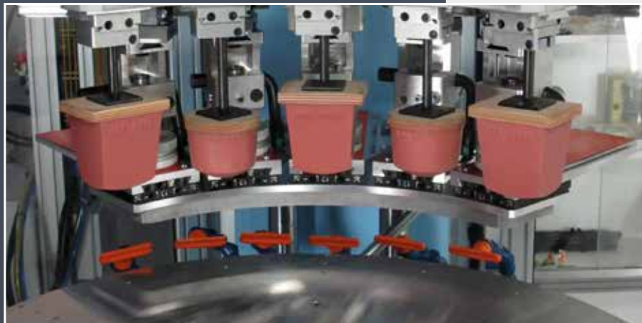
Five colour radial plate configuration with rotary table numerically controlled
